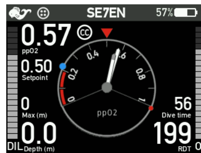
Figure 2-14. Ready-to-dive. At this point, the pre-dive tests are completed, and the system is ready to dive.
