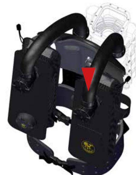
Figure 1-32. Attach the left rear breathing hose to the left counterlung shoulder port.
