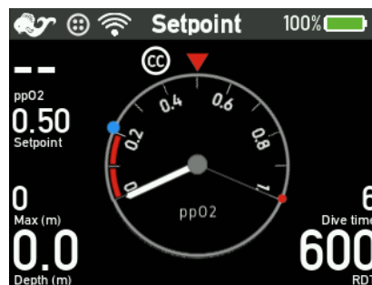
Figure 2-2. Initial display during a few seconds before the M28 enters the PreDiveTest mode, regardless of previous mode.
