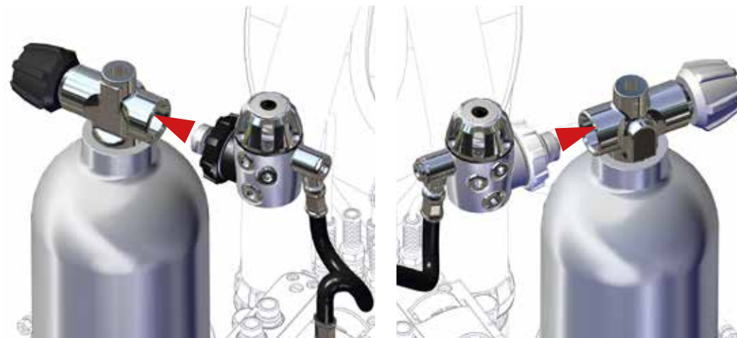
Figure 1-39. Align the diluent regulator with the diluent cylinder female DIN thread. Push it in and hand tighten the diluent regulator swivel nut.
