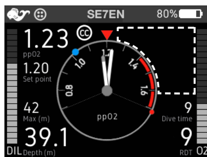
Figure 3-6. Alarm signal area.
