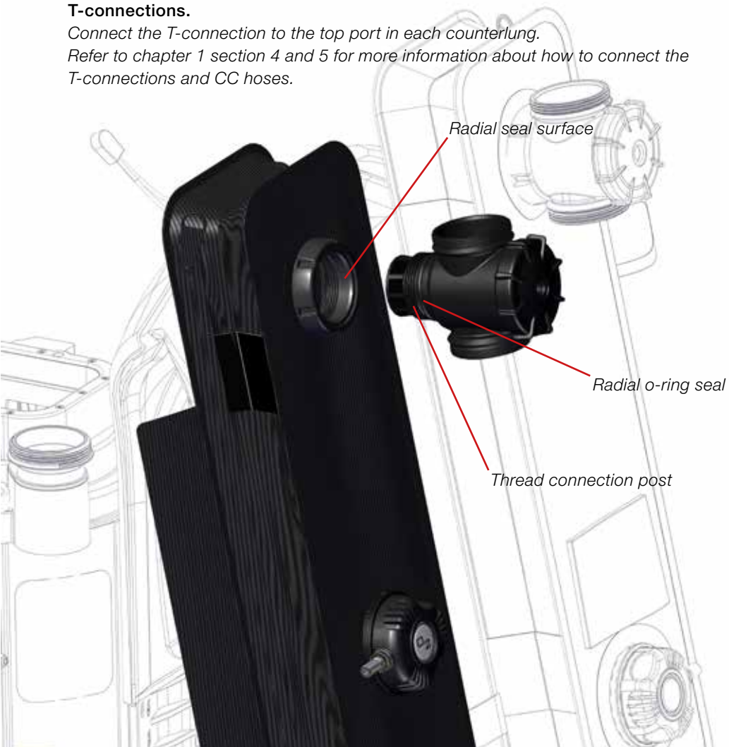
Figure 3-40. Insert the right hand water diversion manifold into the port on the right counterlung. Clockwise tighten the water diversion manifold into the right and left counterlung shoulder port. Note the correct orientation, further described in chapter 1, section 4.
