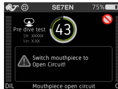
Figure 2-7. Test 43 Switch mouthpiece to OC position, displaying information to the user that the mouthpiece must be placed in the Open-Circuit position.
