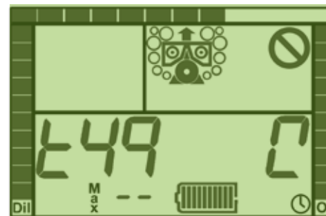
Figure 2-9. Test 49 - Positive pressure loop test.
