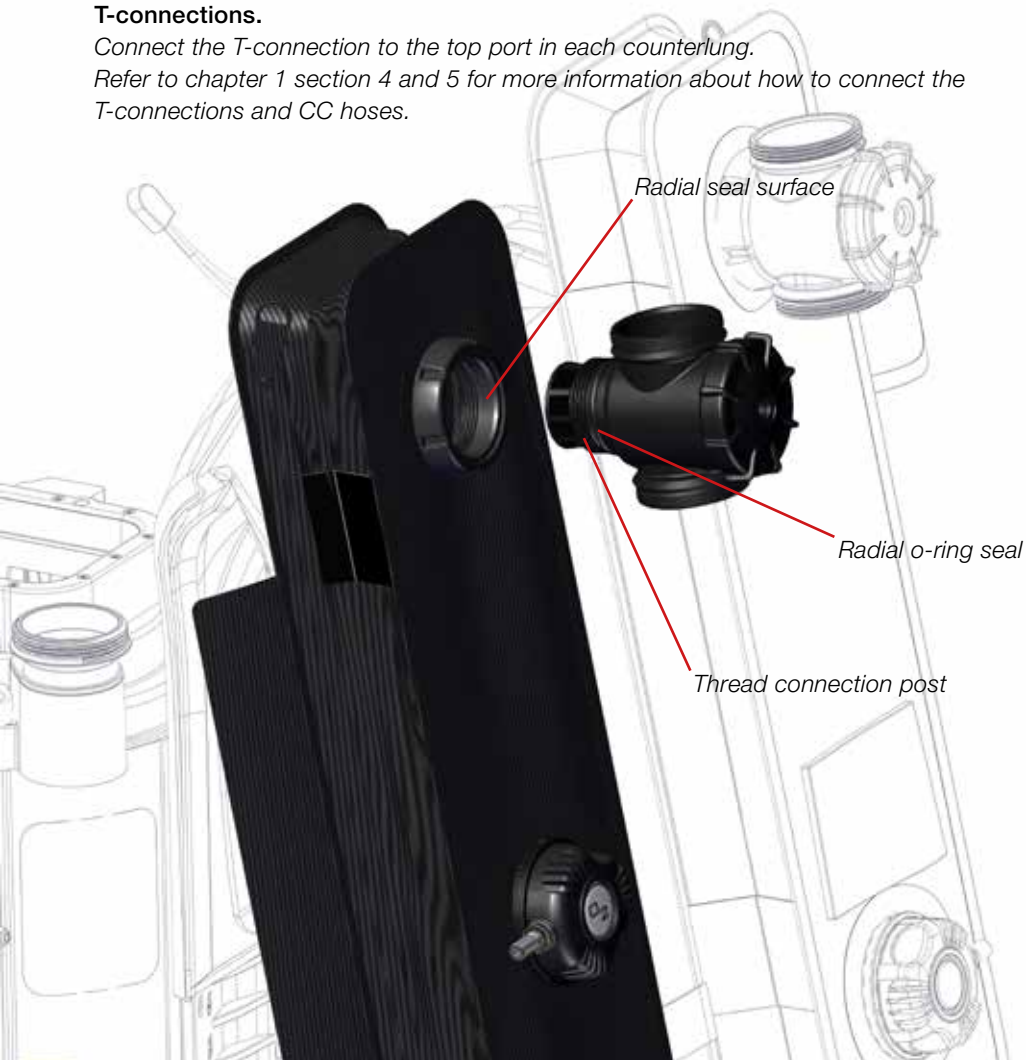
Figure A2-4. Insert the right hand water diversion manifold into the port on the right counterlung. Clockwise tighten the water diversion manifold into the right and left counterlung shoulder port. Note the correct orientation, further described in chapter 1, section 4.
