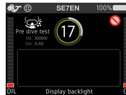
Figure 2-5. Test 17 (Backlight Power consumption), displaying test number in the center circle, progress is shown through the inner green circle moving counter clockwise.
