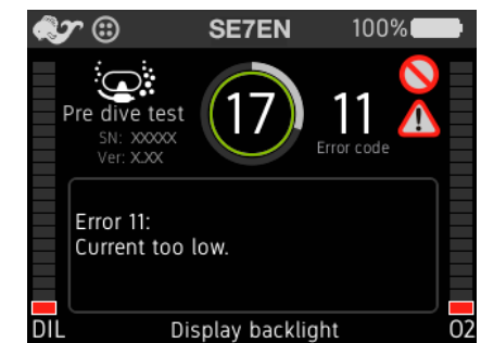
Figure 2-6. Test 17 failure, with flashing error code.
