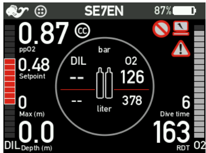
Figure 3-32b. Invalid DIL indicator.
