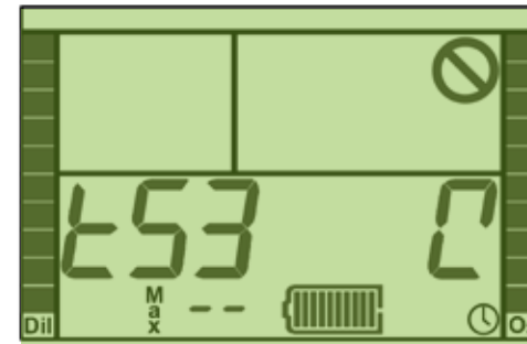
Figure 2-11. Test 53 – Oxygen Sensor calibration.
