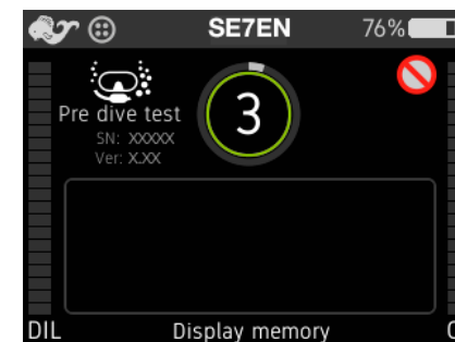
Figure 2-3. PreDiveTest display where the number in the circle represents the test number together with an explanatory text at the bottom of the screen.
