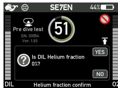
Figure 3-43: Helium confirmation screen at test 51, showing the question of helium fraction content in the diluent gas tank.
