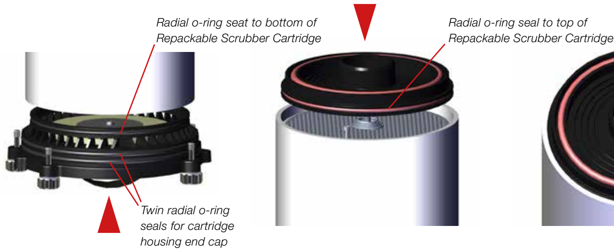
Figure 1-63. Loading the Cartridge End Cap into the new stuffed Repackable Scrubber Cartridge
