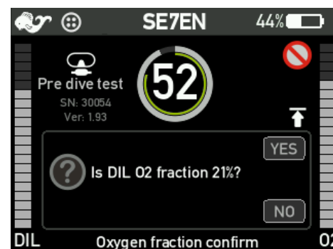
Figure 3-44: Oxygen confirmation screen at test 52, showing the question of oxygen fraction content in the diluent gas tank.
