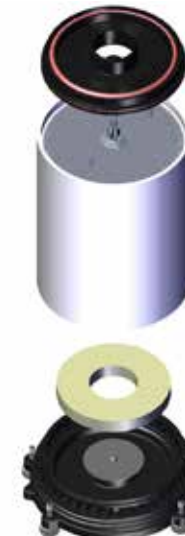
Figure 1-61. Lift and remove the lower sponge; inspect for collected water. Rinse, dry, and store the lower sponge; disinfect if desired.
