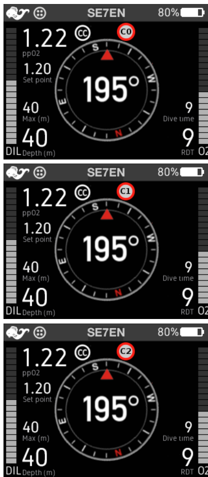
Figure 3-16. Oxygen sensor confidence alerts: C0, C1, C2.
