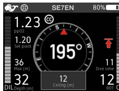
Figure 3-23. Display indicating “ceiling” to which it is safe to ascend & total decompression time.
