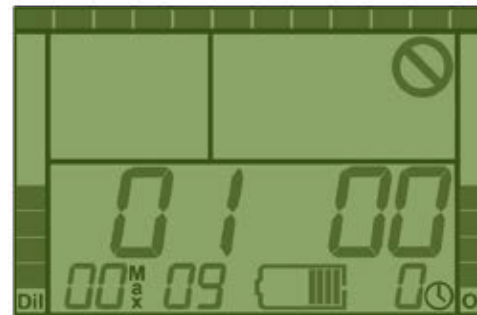
Figure 2-2. Initial displays during the first five seconds of Power-up, showing firmware version and serial number.
