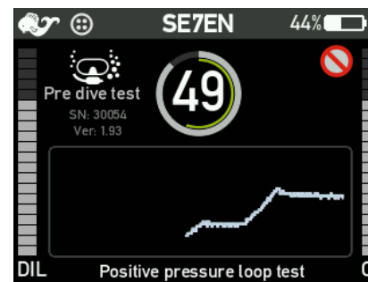
Figure 2-9. Test 49 - Positive pressure loop test.
